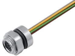
Female panel mount connector, front fastened, with single wires, 8 x 0,14 mm 2
